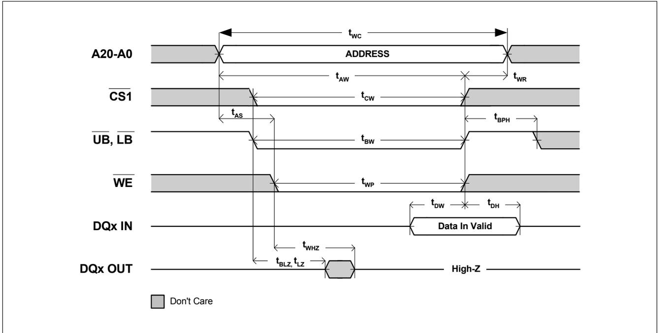
Figure 14 Asynchronous Write -  $\overline{UB}$ ,  $\overline{LB}$  Controlled ( $\overline{OE} = V_{IH}$  or  $V_{IL}$ ,  $\overline{ZZ} = V_{IH}$ )
