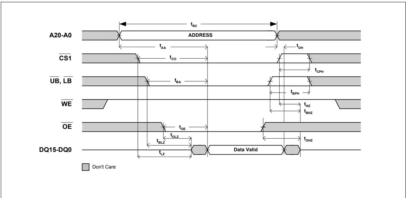
**Figure 10 Asynchronous Read ( $\overline{WE} = V_{IH}$ ,  $\overline{ZZ} = V_{IH}$ )**
