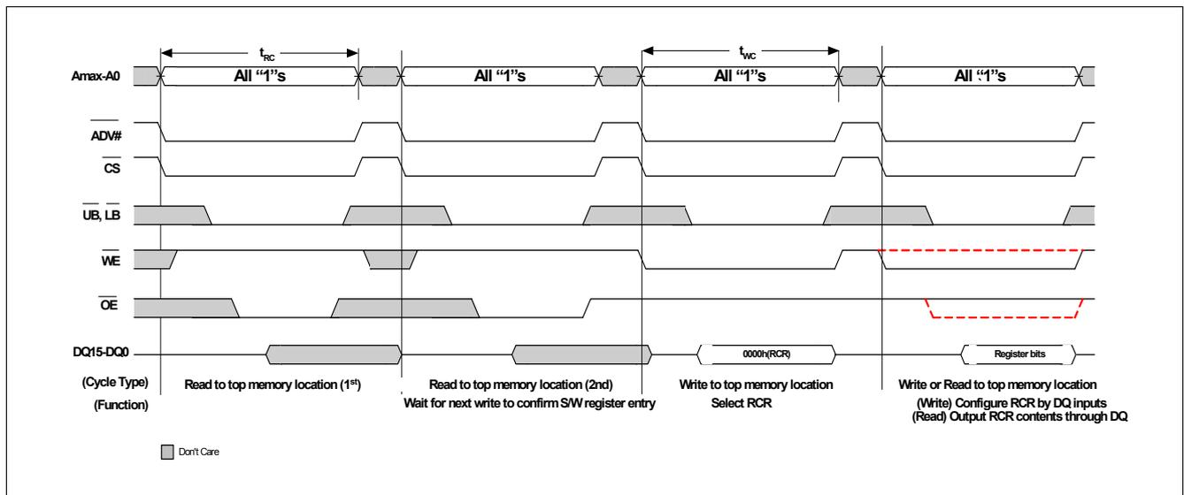
Figure 19 S/W Register Entry timing (Address input = 1FFFFh)
