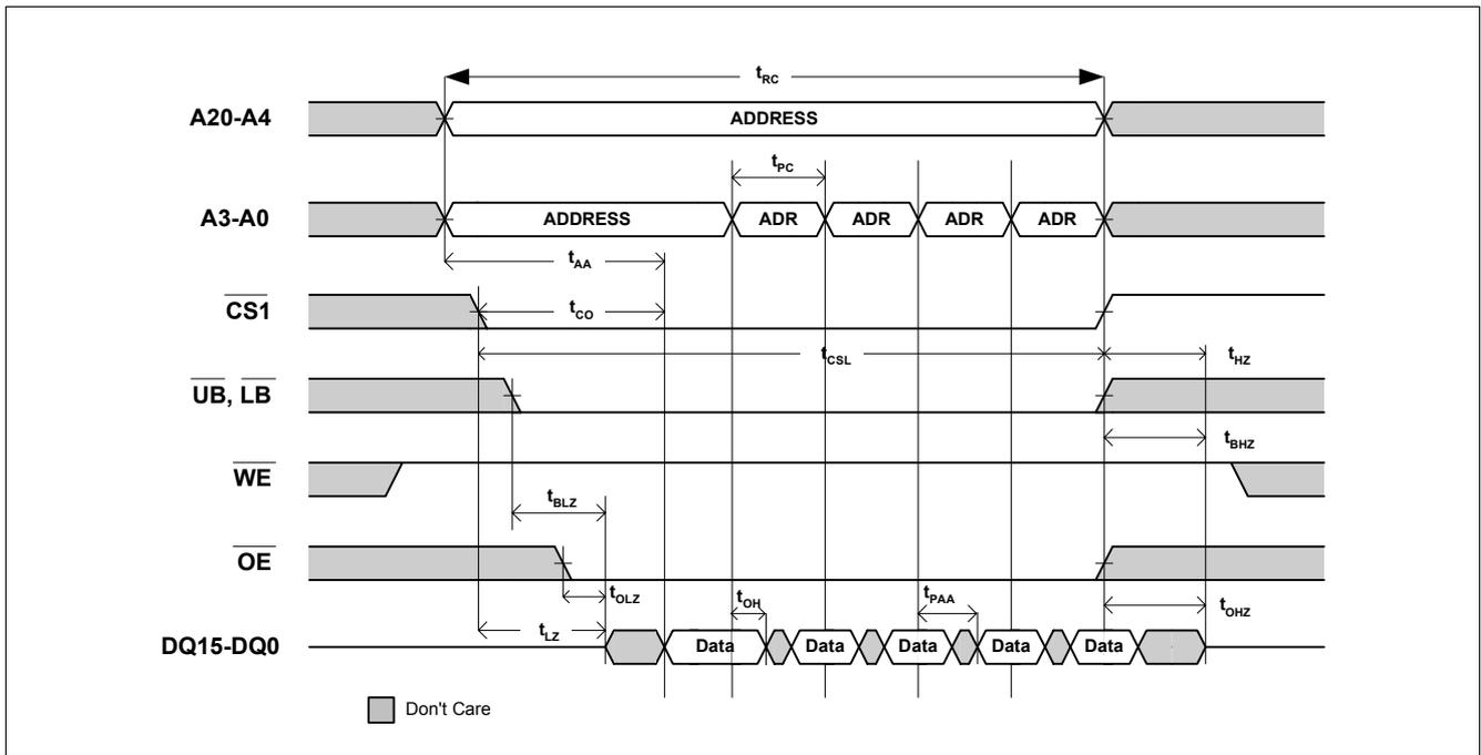
Figure 11 Asynchronous Page Read Mode ( $\overline{ZZ} = V_{IH}$ )
