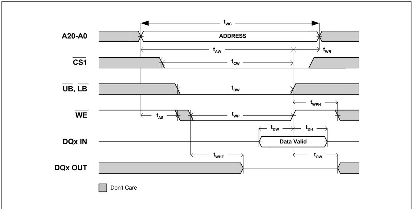
Figure 12 Asynchronous Write -  $\overline{WE}$  Controlled ( $\overline{OE} = V_{IH}$  or  $V_{IL}$ ,  $\overline{ZZ} = V_{IH}$ )
